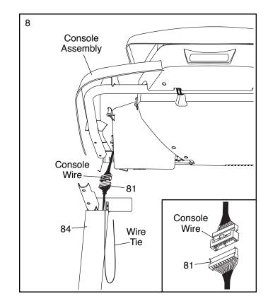
9. Set the console assembly on the Right and Left Handrails (84, 85). **Make sure that no wires are pinched.** Insert the excess Upright Wire (81) into the Right Upright (90).
