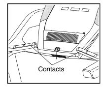
To measure your heart rate, stand on the foot rails and hold the pulse bar with your palms on the contacts; avoid moving your hands. When your pulse is detected, several dashes will appear in the display and then your heart rate will be shown. For the most accurate heart rate reading, continue to hold the contacts for about 15 seconds.
