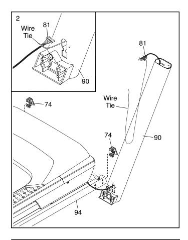
3. Lay the Right Upright (90) near the Base (94). Press the Grommet (77) into the square hole in the Right Upright. Make sure not to pinch the ground wire.
