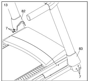
14 .Note: If it is assembled on a smooth surface, the treadmill may roll forward during this step.
